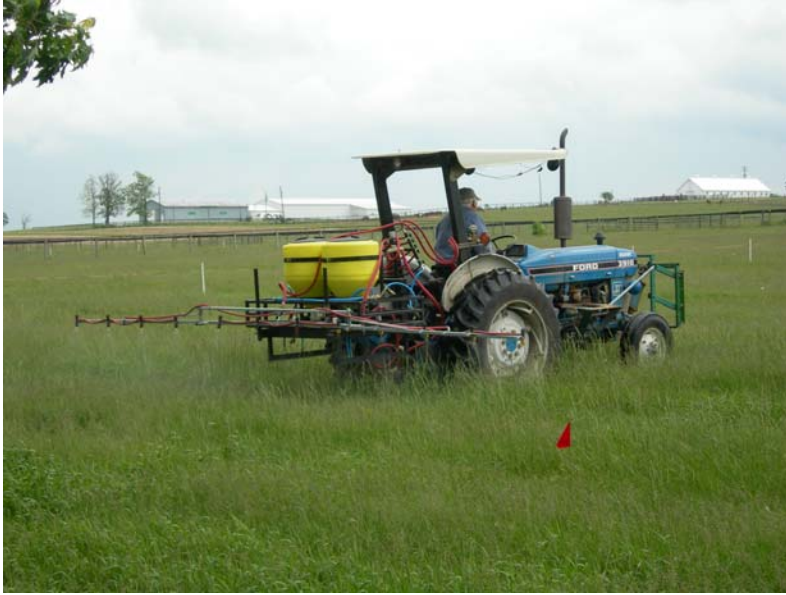
Figure 2.1. A CO 2 pressurized plot sprayer was used to apply the assigned treatments in the Spring 2005 through Fall 2006 studies.
