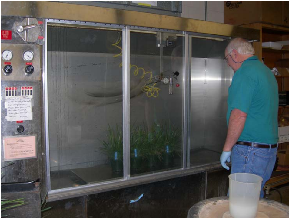
Figure 3.2. Dr. William W. Witt operating the research track sprayer. This machine applied the Cimarron® and Plateau® treatment to the E+ fescue pots at a rate and concentration equivalent to those used in Experiment 1.
